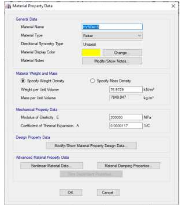
Fig. 6: Defining Properties of Rebar
