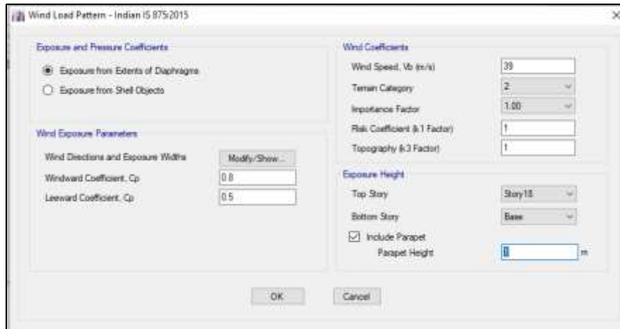
Fig. 16: Wind Load Pattern as per IS 875:2015.
