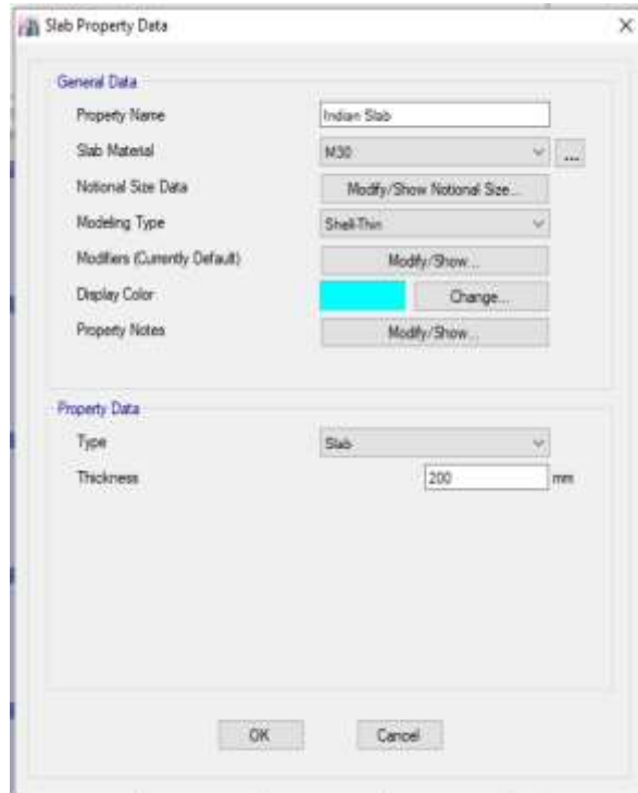
Fig. 13: Defining Properties of Slab
