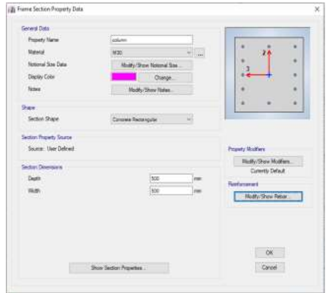
Fig. 10: Defining section properties of Column
