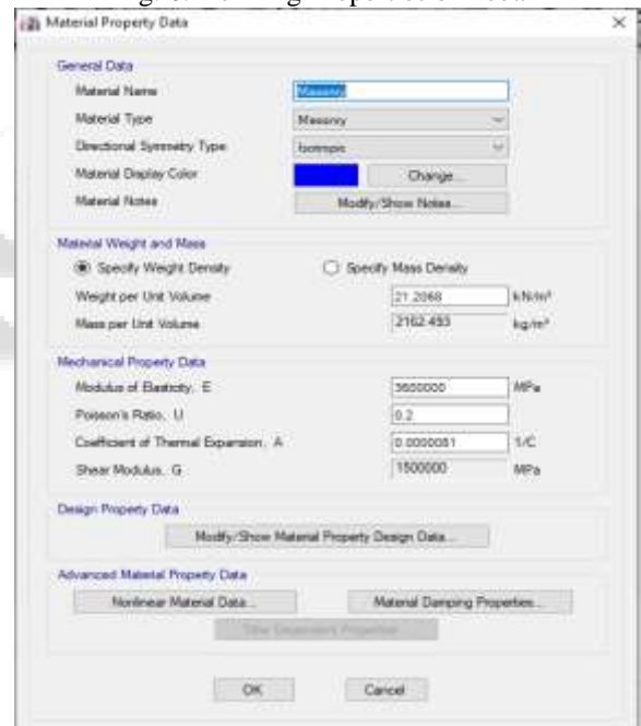
Fig. 7: Defining Properties of Masonry
