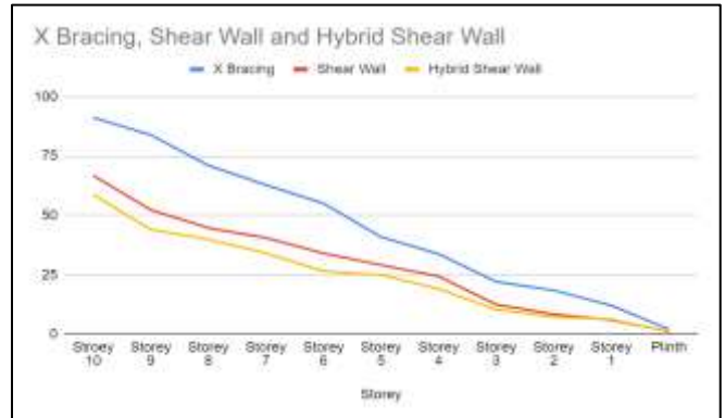
Fig. 20: Storey Displacement in mm
