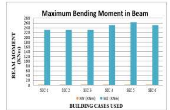
Fig. 11: Maximum Shear Forces and Bending Moments in Beam for all Stability Improving Cases
