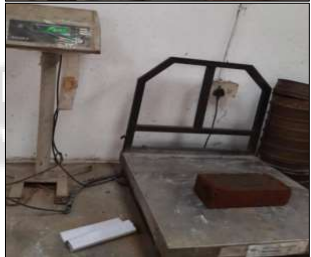
Fig. 12, 13: Water Absorption Test
