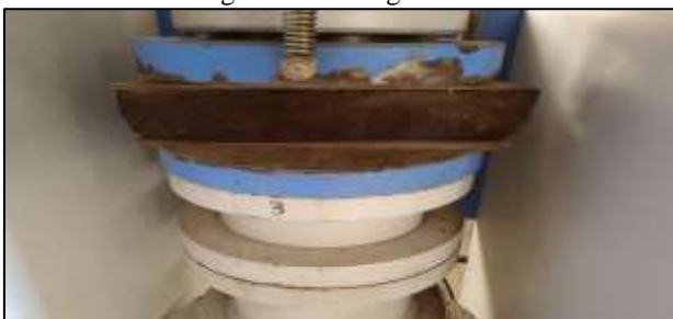
Fig. 4: Compressive Strength of cow Dung Bricks
