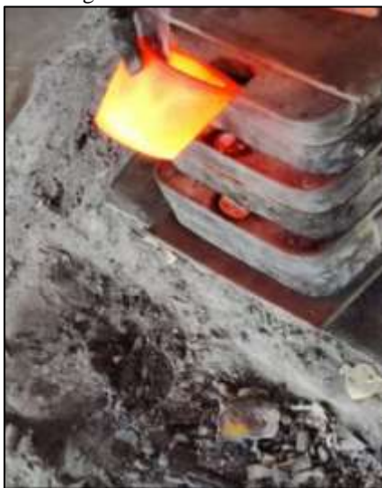
Fig. 1: Graphite crucible in sand casting process
