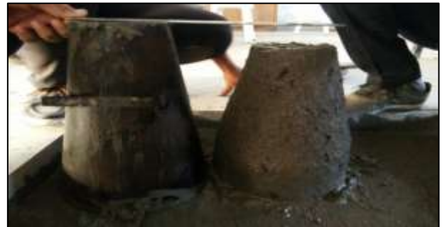
Fig. 3.2.3.3: Workability test by using slump cone
