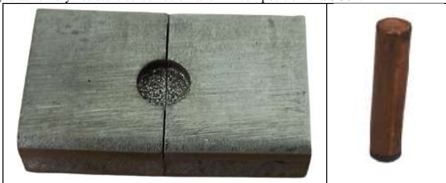
Fig 3: Work piece (304 Stainless Steel) and Tool (Cylindrical Copper Electrode)
