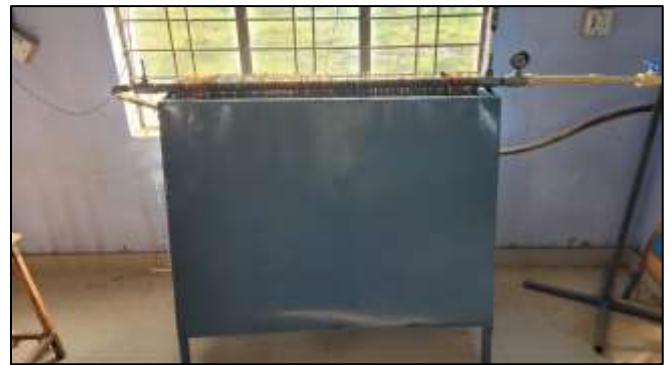
Fig. 4: physical set up for heat exchanger with internal grooving with rectangular fin.
