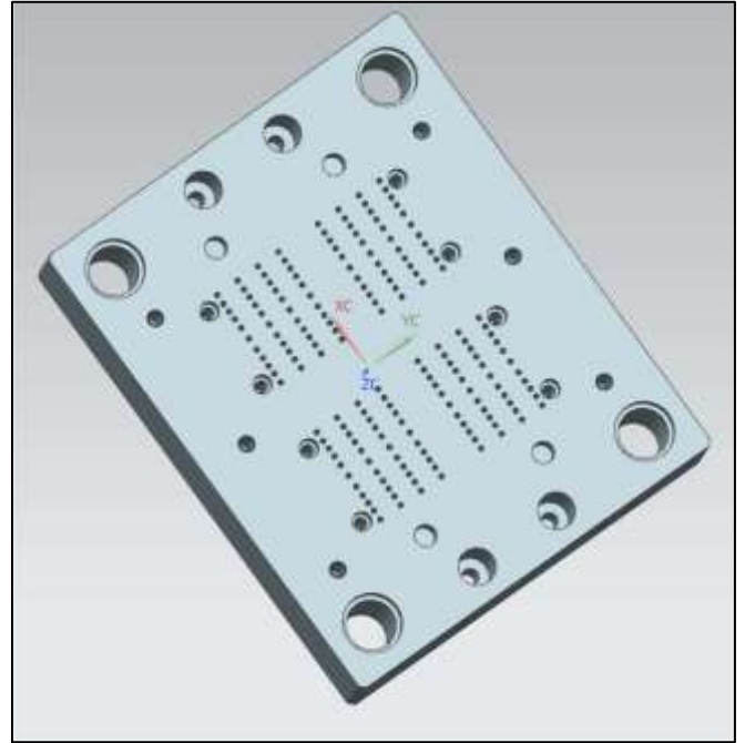
Fig. 21: Core Housing 3D Bottom View
