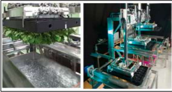
Fig. 3: Automated modules for upside-down vacuum and infiltration [19]
