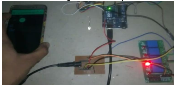
Fig. 7: LED on Relay unit glows when Pump is turned “On”.
