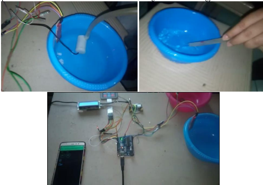
Fig. 8: Final Interfacing of Arduino with Pump.
