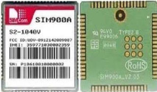
Fig. 6: GSM Module
