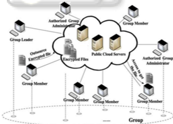
Fig. 1: An Example of Cloud based group Sharing Scenario Fig. 1 for example, the normal group application scenario in cloud can be described as follows: The group leader opens up a sharing area in the cloud to form a group application.
