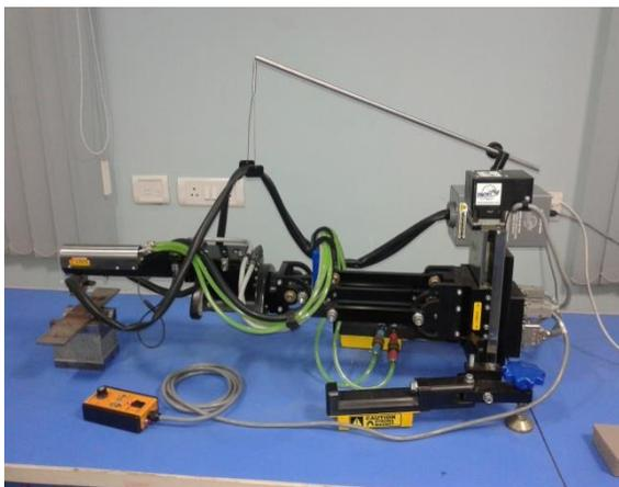
Fig. 2: Equipment of X-Ray Diffraction
