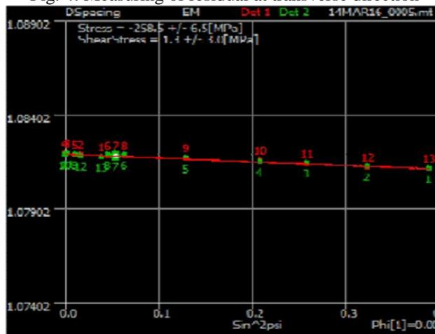
Fig. 5: A linear graph of d vs.  $\sin^2\psi$  fitted to diffraction data with a negative slope
