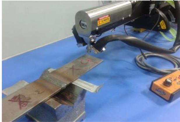
Fig. 4: Measuring of residual at transverse direction
