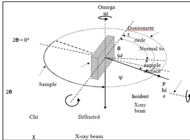
Fig. 1: Angles and rotations used in residual stress measurement
