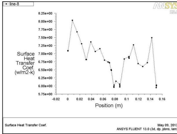
Fig. 12: Variation of Surface heat transfer coefficient along the length of the pipe
