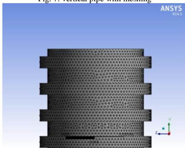
Fig. 8: vertical pipe with rectangular fins after meshing
