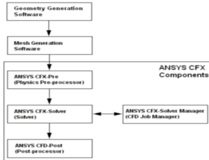
Fig. 1: Block Diagram of ANSYS simulation
