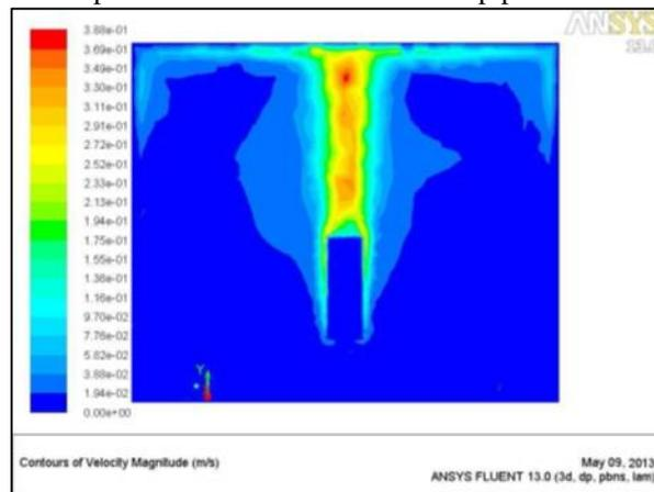
Fig. 15: Velocity Counters Of Circular Pipe without Fins
