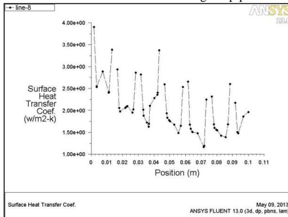
Fig. 21: variation of Surface heat transfer coefficient along the pipe with triangular fins
