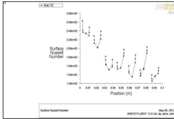
Fig. 25: Variation of Surface Nusselt number along the pipe with Trapezoidal fins
