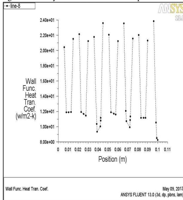
Fig. 16: Variation of Surface heat transfer coefficient along the length of the pipe
