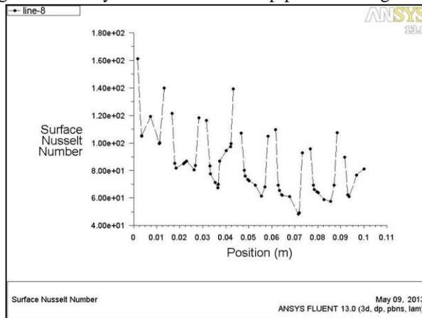
Fig. 20: variation of Surface Nusselt number along the pipe with triangular fins
