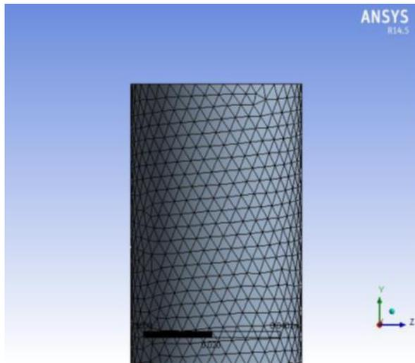
Fig. 7: vertical pipe with meshing
