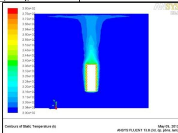
Fig. 18: The temperature contours of the circular pipe in case of triangular fins
