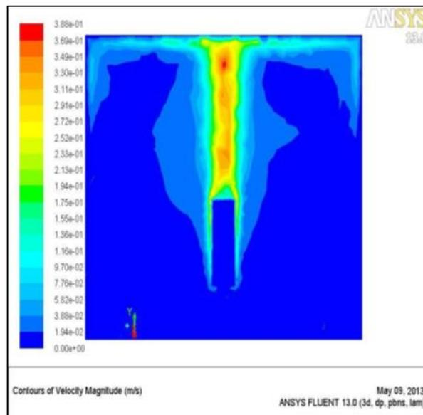
Fig. 11: Velocity Counters Of Circular Pipe without Fins
