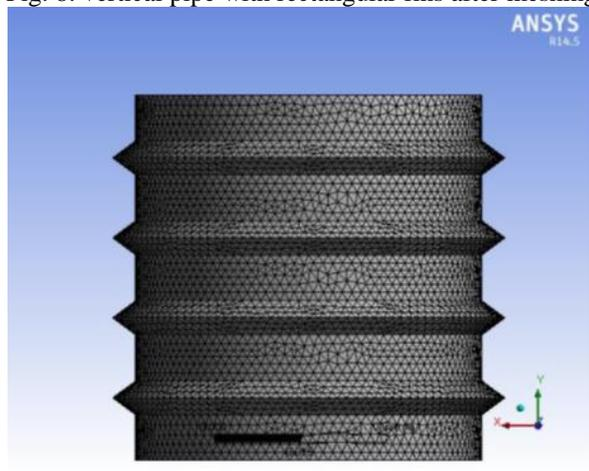
Fig. 8: vertical pipe with triangular fins after meshing
