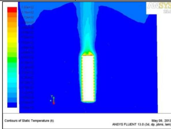
Fig. 22: The temperature contours of the circular pipe with Trapezoidal fins
