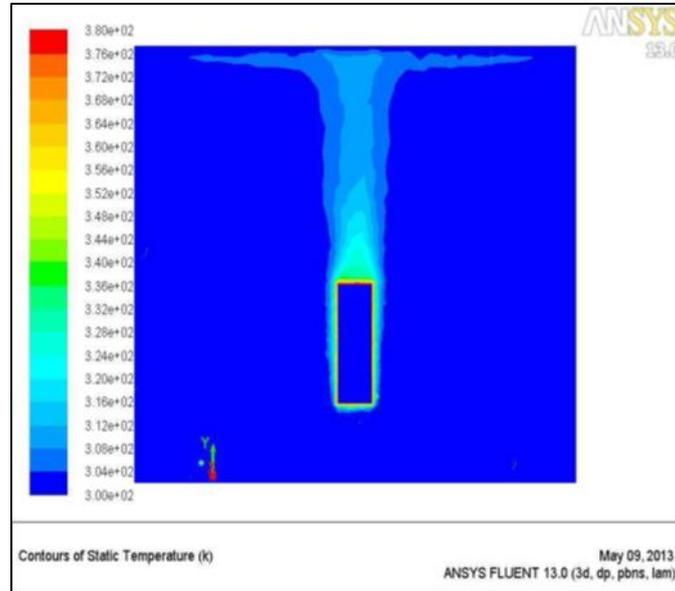
Fig. 10: Temperature contours of the circular pipe without fins
