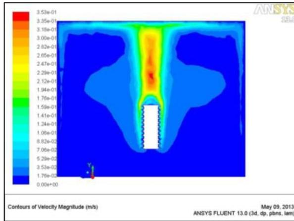
Fig. 19: Velocity counters of circular pipe with triangular fins
