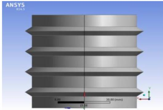
Fig. 4: Vertical Pipe with Triangular Fin
