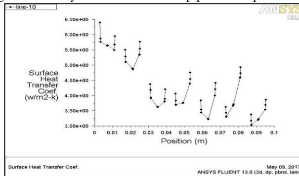
Fig. 24: The variation of Surface heat transfer coefficient along pipe with Trapezoidal fins
