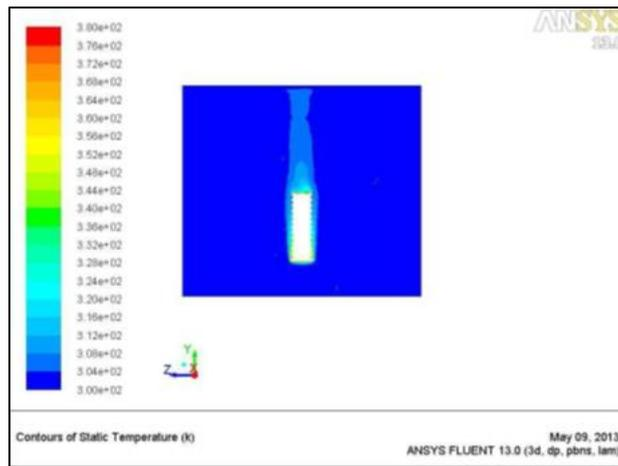
Fig. 14: The temperature contours of the circular pipe with rectangular fins
