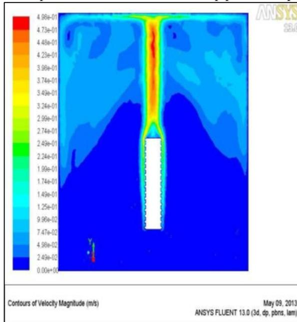
Fig. 23: Velocity counters of circular pipe with trapezoidal fins
