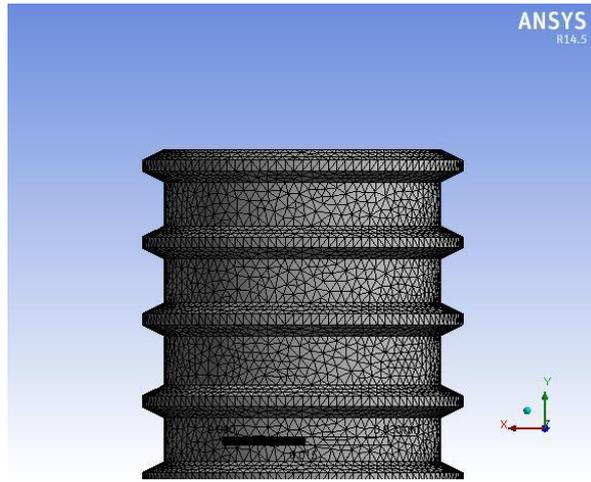
Fig. 9: vertical pipe with trapezoidal fins after meshing
