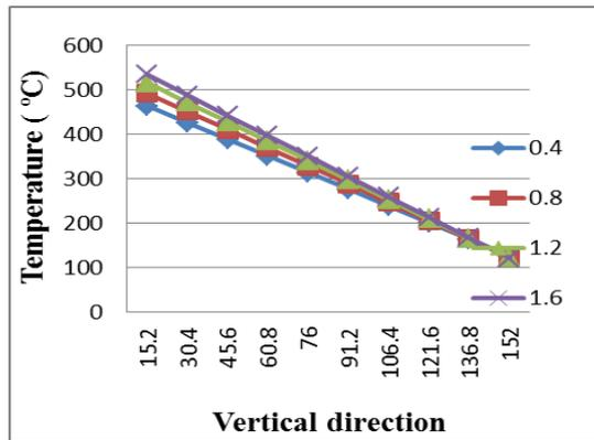
Fig. 16.1: Variation of temperature in the ceramic coated piston ( $MgZrO_3$  &  $NiCrAl$ ) in vertical direction for different coating thickness
