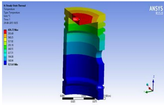
Fig. 5: Variation of temperature in the piston without coating
