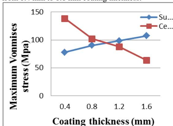
Fig. 22: Variation of maximum vonmises stress in the substrate and ceramic coated piston with different coating thickness
