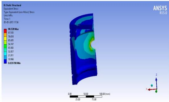
Fig. 11: With 1.2 mm coating thickness
