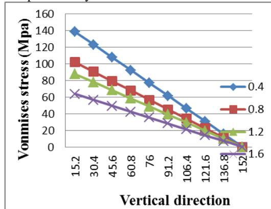
Fig. 20: Variation of vomises stress in the ceramic coated piston (Mgzro<sub>3</sub> & NiCrAl) in vertical direction for different coating thickness
