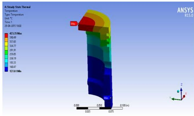
Fig. 7: With 0.8mm Coating Thickness
