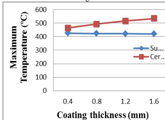
Fig. 21: Variation of maximum temperature in the substrate and ceramic coated piston with different coating thickness
