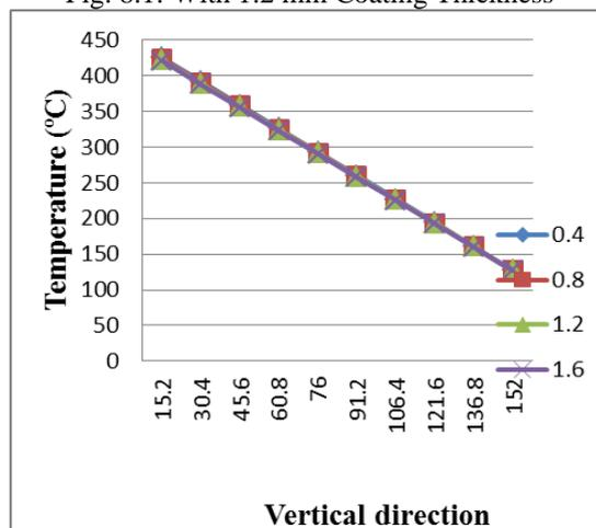
Fig. 8.2: Variation of temperature in the piston (substrate) in vertical direction for different coating thickness
