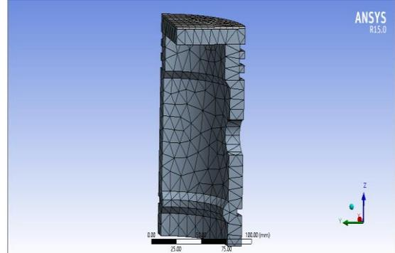
Fig. 4: Meshed quarter part of the piston with coating
