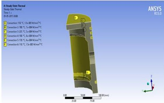
Fig. 3: Piston model with various thermal boundary conditions
