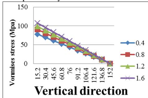
Fig. 12.1: Variation of maximum temperature and maximum thermal stresses in the piston (substrate) with coating thickness
