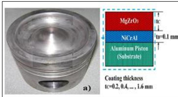
Fig. 2: The piston used in the FE analyses: a) photograph of the piston used diesel engine, b) the coating parameters
