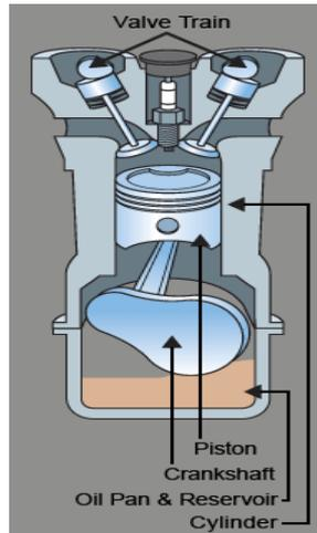
Fig. 3: Single Piston Cylinder
