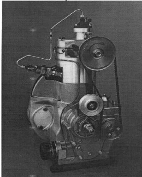
Fig. 1: Prototype of 6-stroke engine
