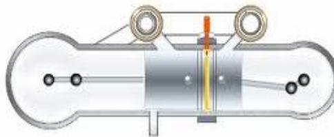
Fig. 4: Opposed piston cylinder
