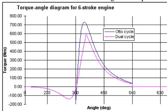
Fig. 7: Torque angle diagram for 6 stroke engine
