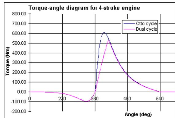
Fig. 8: Torque angle diagram for 4 stroke engine
