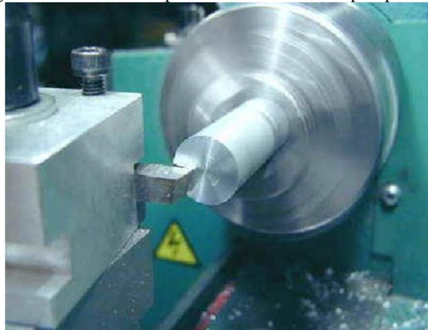
Fig. 4: Facing and Turning Operations
