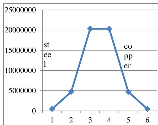
Fig. 8: Gaussian heat distribution, X-Axis: Distance (mm) Y-Axis: Heat Flux ( )
