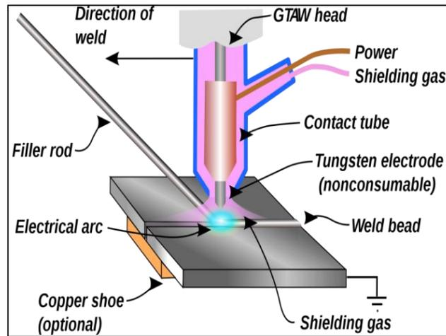
Fig. 1: Tig Welding process
