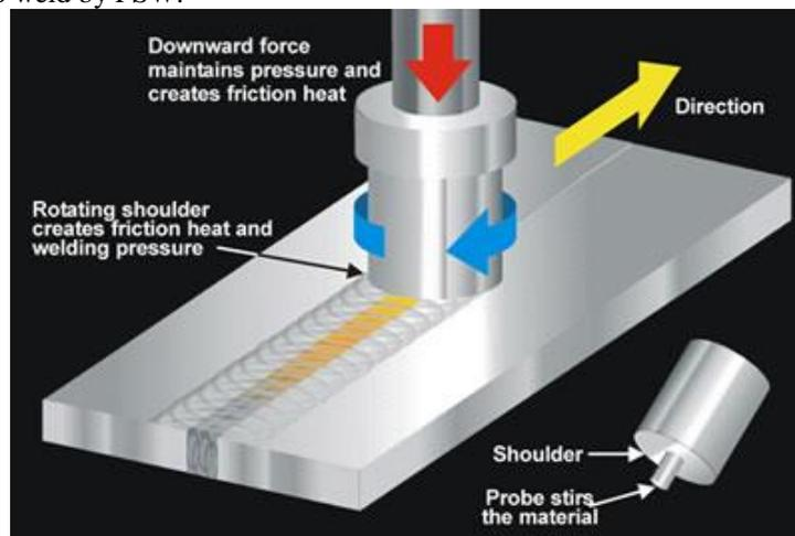
Fig. 1: Friction Stir Welding
