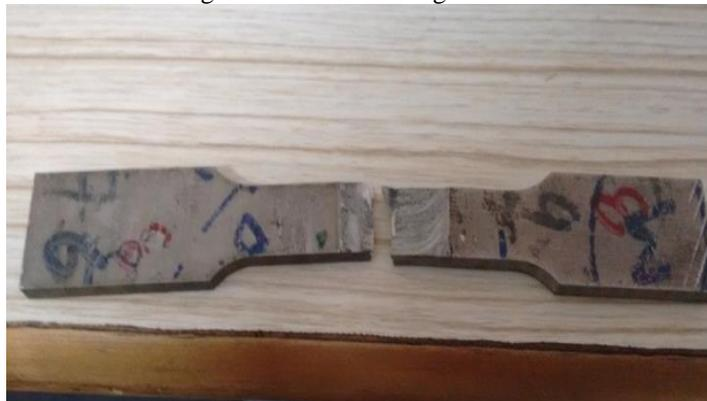
Fig. 9: Broken Test Piece
