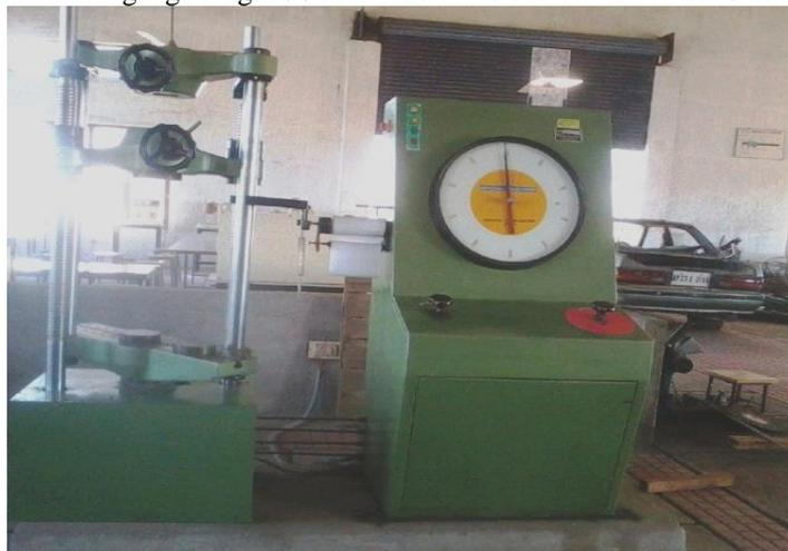
Fig. 8: Universal Testing Machine
