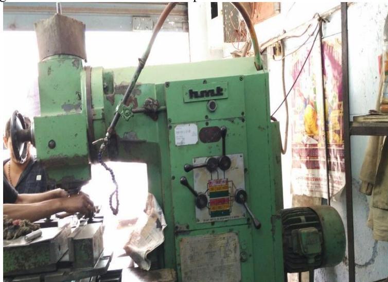
Fig. 6: 4-Axes Milling Machine
