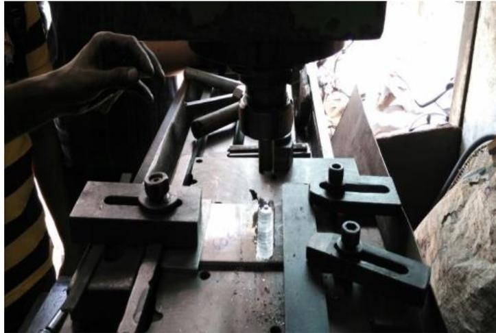
Fig. 7: Friction stir welding process
