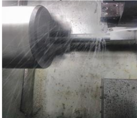
Fig. 7: Machining of Work Piece EN 353 Alloys with SAE 40+ Boric Acid
