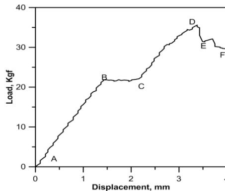
Fig. 4: Load vs Displacement data for flexural strength test in longitudinal orientation
