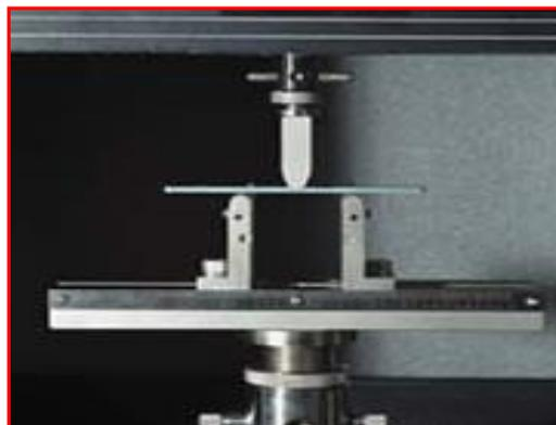
Fig. 3: Three Point Bending Test Setup
