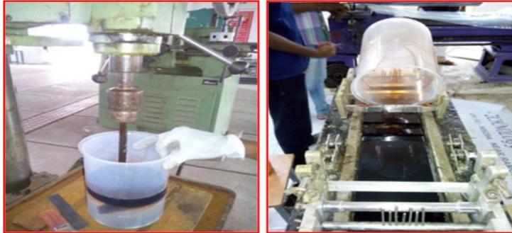
Fig. 1: Resin mixing and Creel Stand
