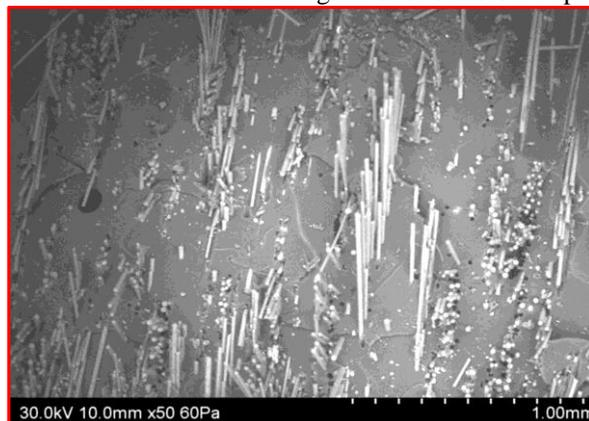
Fig. 5: SEM Fractograph of glass fiber reinforced epoxy matrix composite
