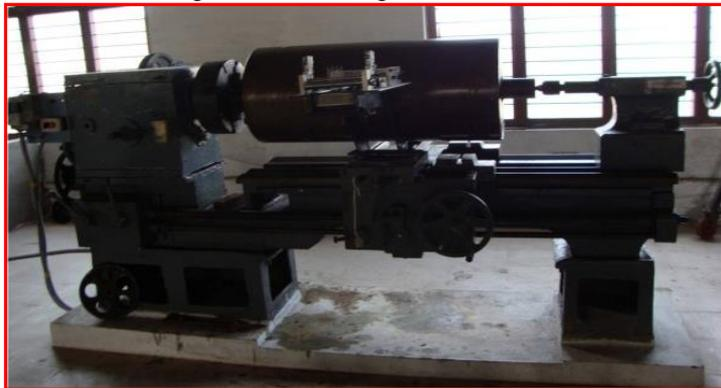
Fig. 2: Filament Winding Machine
