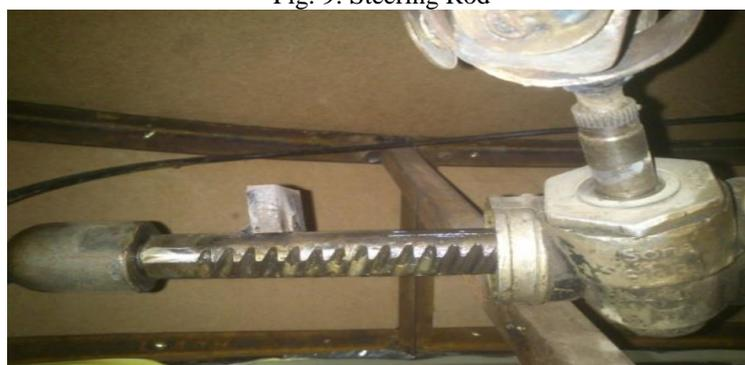
Fig. 10: Steering Gear Rack and Pinion
