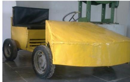
Fig. 12: Car Body with Al Sheet
