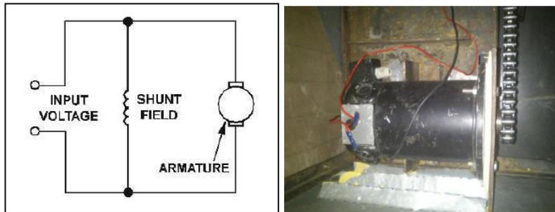
Fig. 7: Shunt Motor
