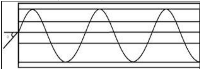
Fig. 1: Path followed by the ray in graded optic fibre
