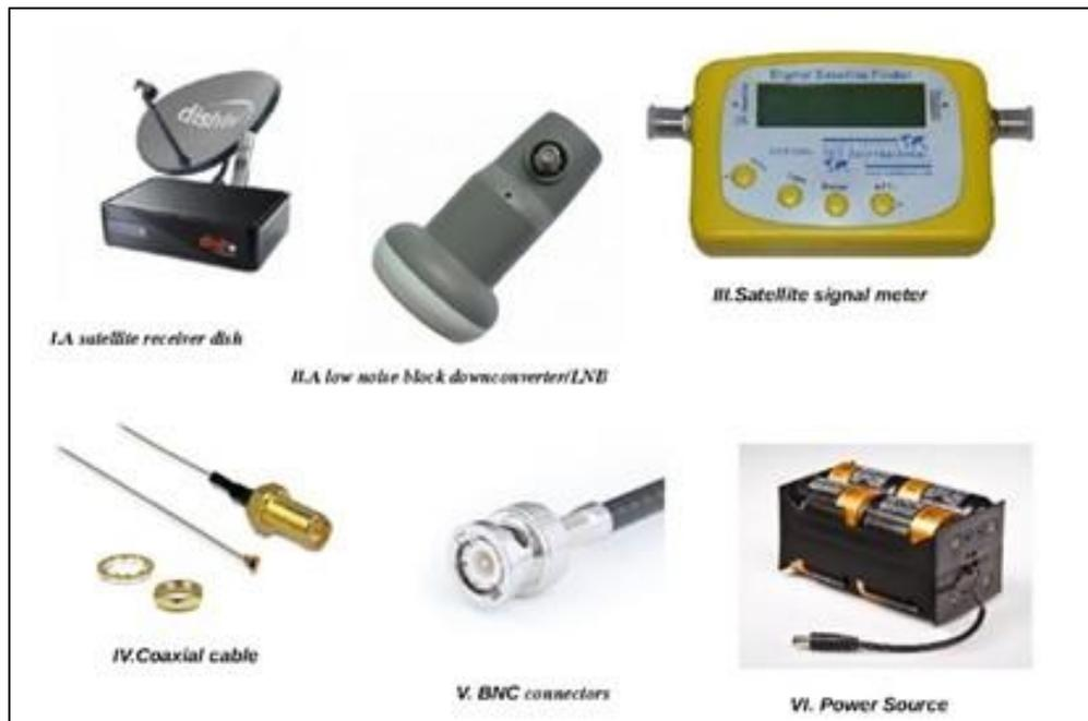
Fig. 1: Material required for constructing Radio Telescope mostly available on e-markets.
