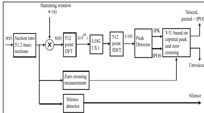
Fig. 1: Block diagram of Cepstrum pitch detector
