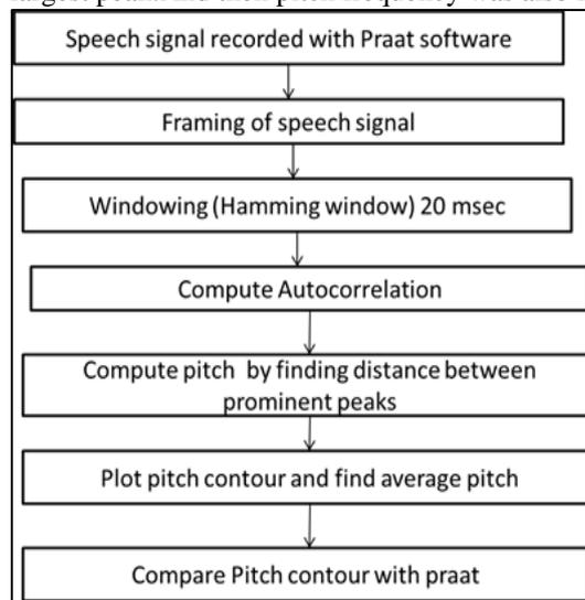
Fig. 5: Algorithm of Autocorrelation
