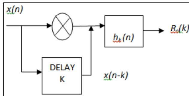
Fig. 4: Block Diagram Representation of short time autocorrelation[1]
