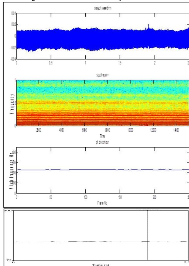
Fig. 6: Pitch contour from autocorrelation algorithm and Praat software for /a/ vowel. (a)Speech waveform (b) spectrogram of speech signal (c) Implemented autocorrelation pitch estimation (d) Pitch estimation by Praat software
