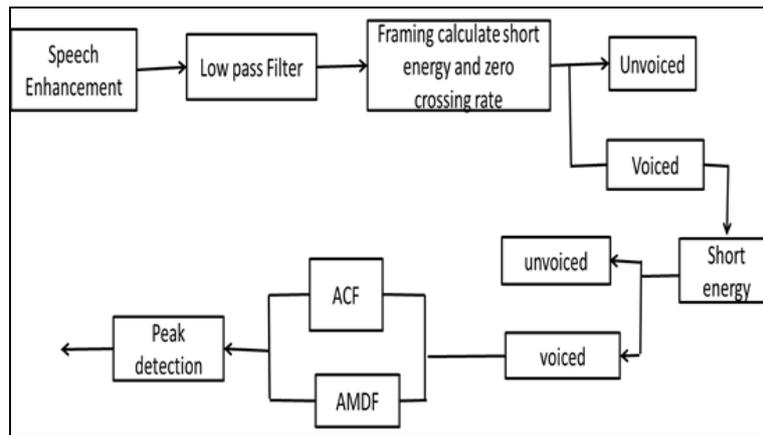
Fig. 3: Flow diagram of pitch detection [9]
