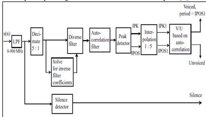
Fig. 2: Block diagram of SIFT pitch detector
