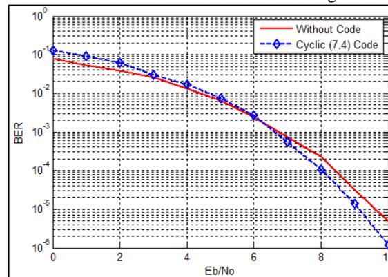
Fig. 6: Performance comparison without error correcting codes, with Cyclic (7, 4) Codes
