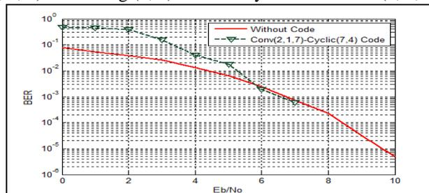
Fig. 9: Performance comparison without error correcting codes, with Concatenated Convolutional (2, 1, 7) -Cyclic (7, 4) codes
