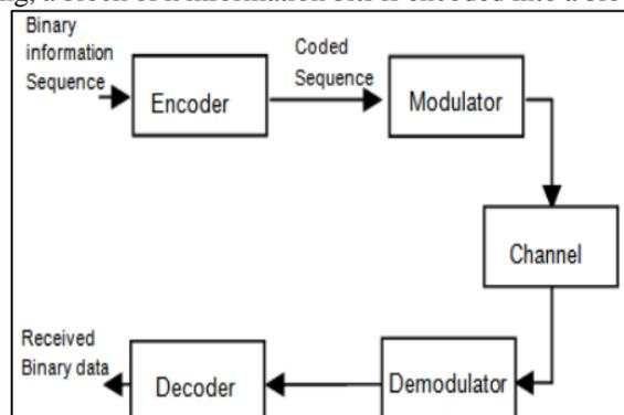
Fig. 1: Generic Block diagram of digital communication system
