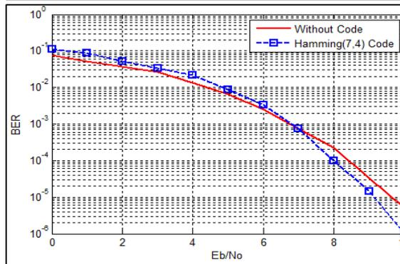
Fig. 5: Performance comparison without error correcting codes, with Hamming (7,4) codes
