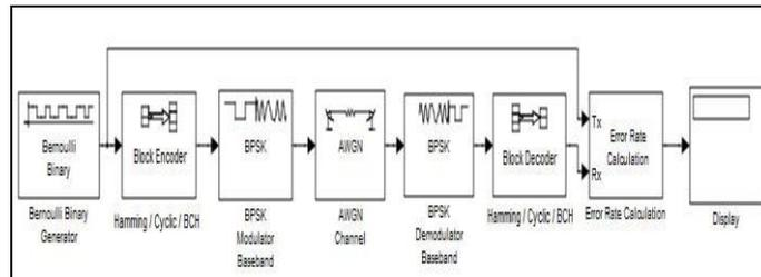
Fig. 3: Simulation with Hamming, Cyclic and BCH Error Correcting Codes
