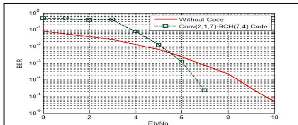
Fig. 10: Performance comparison without error correcting codes, with Concatenated Convolutional (2, 1, 7) -BCH (7, 4) codes
