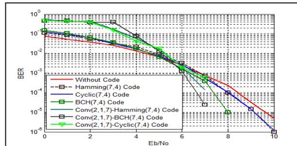
Fig. 11: Performance comparison without error Correcting Codes, with Hamming (7, 4), Cyclic (7, 4), BCH (7, 4), Convolutional (2, 1, 7)-Hamming (7, 4), Convolutional (2, 1, 7)-BCH (7, 4) codes, Convolutional (2, 1, 7)-Cyclic (7, 4)
