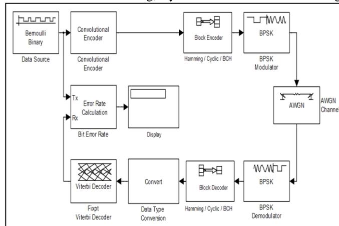
Fig. 4: Simulation with Concatenated Error Correcting Code
