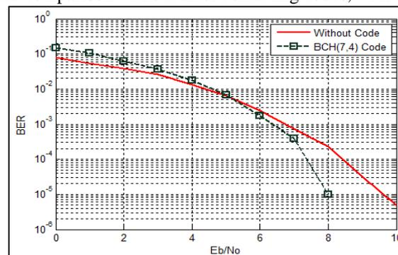
Fig. 7: Performance comparison without error correcting Codes, with BCH (7, 4) codes
