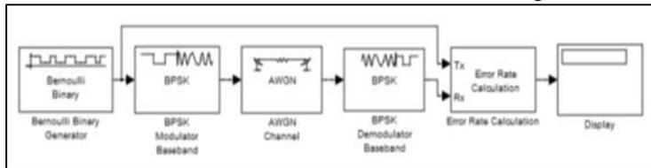
Fig. 2: Simulation without Error Correcting Codes
