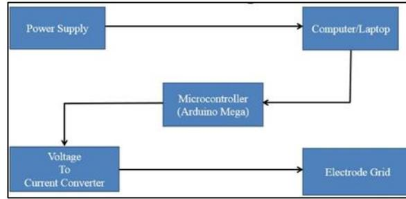
Fig. 3: Block Diagram of Electronic Braille Reader
