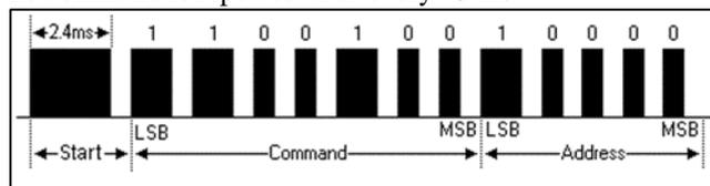
Fig. 5: SONY SIRC Protocol
