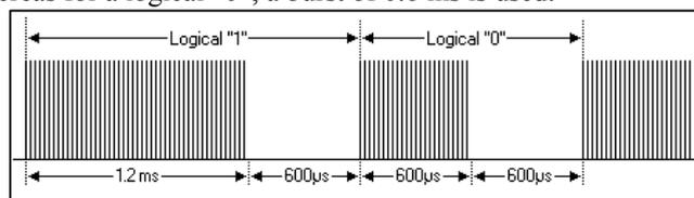
Fig. 4: SONY SIRC Modulation
