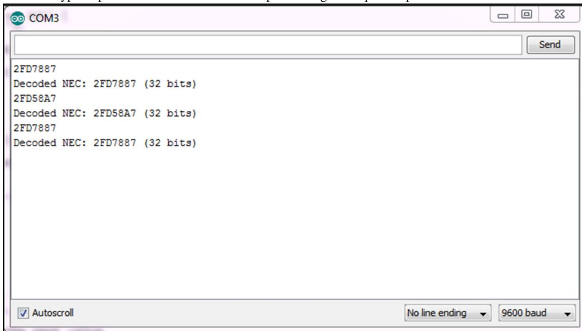
Fig. 8: Decoded Output for NEC (Volume Up and Down)
