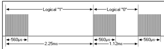
Fig. 2: NEC Modulation
