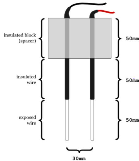
Fig. 3: Soil moisture detector
