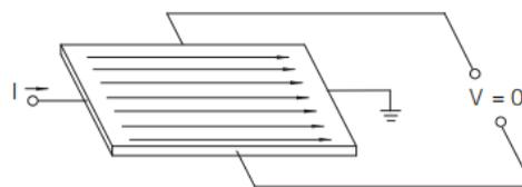
Fig. 5: Hall effect principle, no magnetic field
