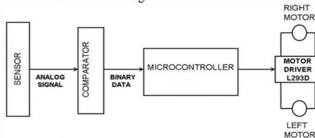
Fig. 4: Basic block diagram of Farm bot
