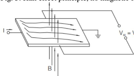
Fig. 6: Hall effect principle, when magnetic field is present
