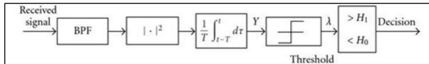
Fig. 3: Block diagram of energy detection.
