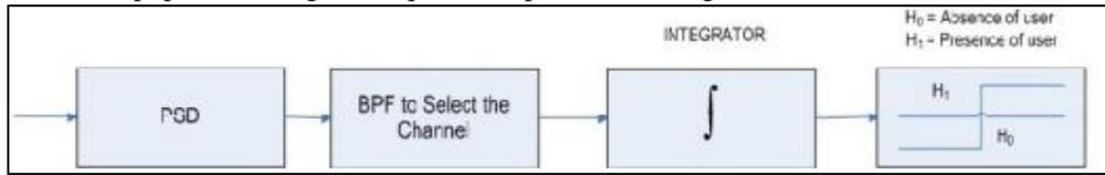
Fig. 2: Energy detector block diagram.
