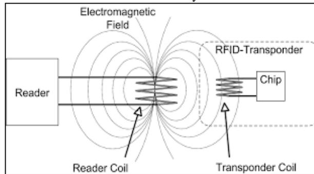
Fig. 2: RFID Basic Functioning
