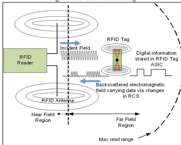
Fig. 3: RFID Communication
