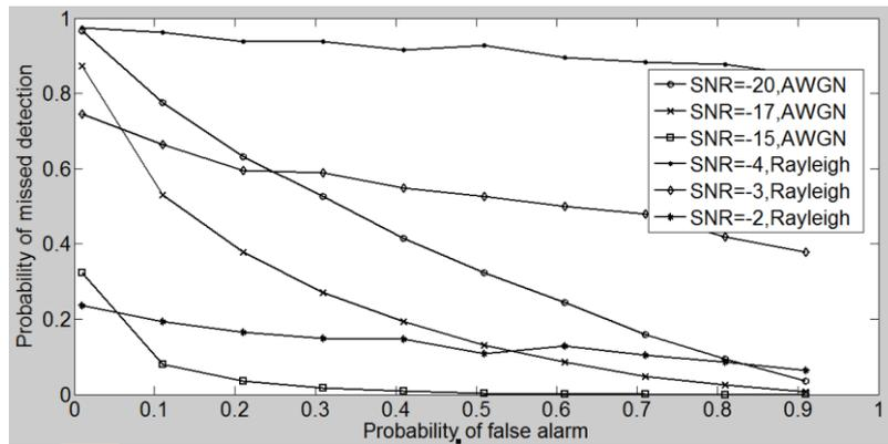
Fig. 11: Probability of false alarm versus probability of missed detection
