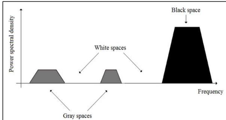
Fig. 2: Spaces in radio spectrum [6]
