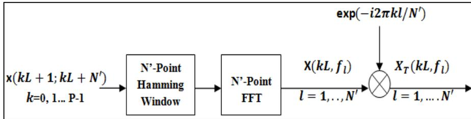
Fig. 7: Cyclostationary based detector [13]
