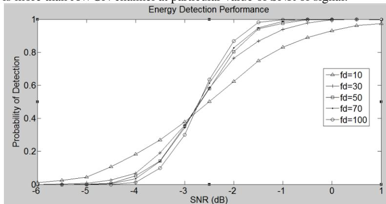
Fig. 12: SNR versus probability of detection for Rayleigh fading channel
