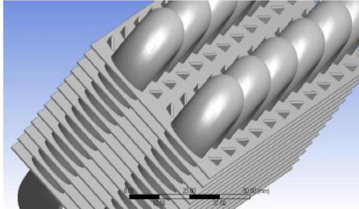
Fig. 4: Enlarged view of finned tube heat exchanger with vortex generator
