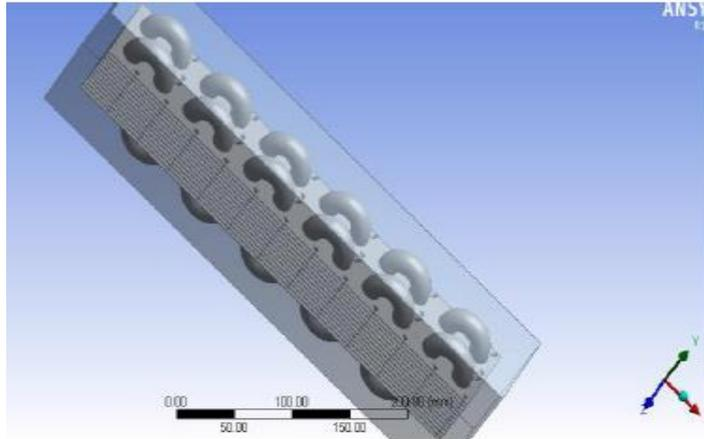
Fig. 3: Schematic view of finned tube heat exchanger with vortex generator
