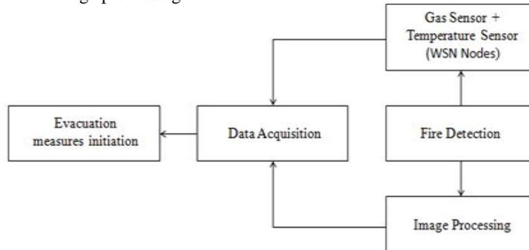
Fig. 1: Block diagram of the Detection and Evacuation Technique
