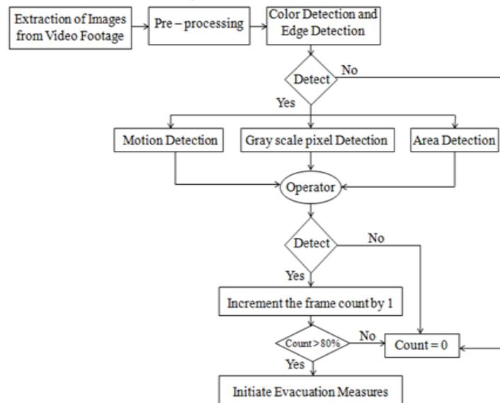
Fig. 4: Process flow of image processing unit
