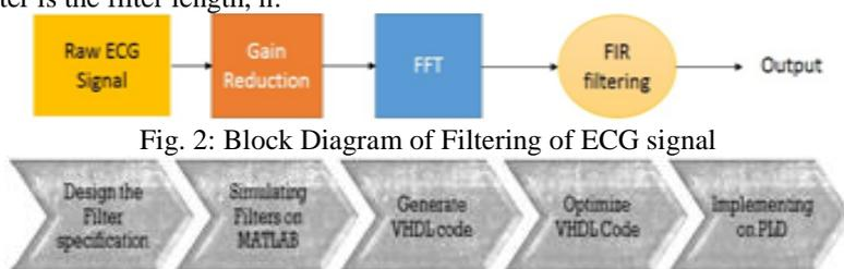
Fig. 2: Block Diagram of Filtering of ECG signal
