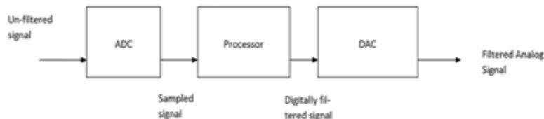
Fig. 1: Block Diagram of general signal processing system
