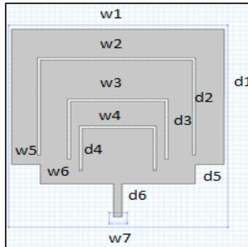
Fig. 1: Antenna Geometry
