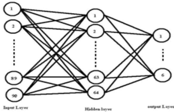
Fig. 4: Architecture of Neural Network
