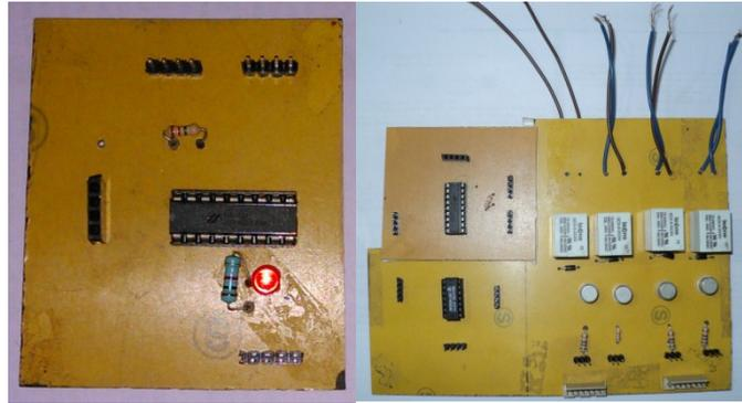
Fig. 6: Original view of Transmitter circuit Fig. 7: Original view of Receiver & Driver circuit
