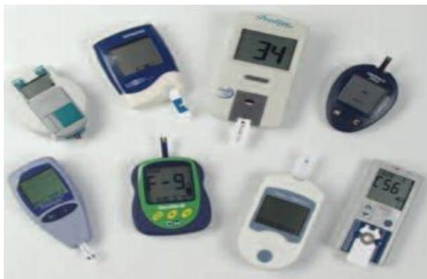
Fig. 2: With the 21st century came a number of different electrochemical glucose meter systems, including the OneTouch Ultra (top right) from Johnson & Johnson.
