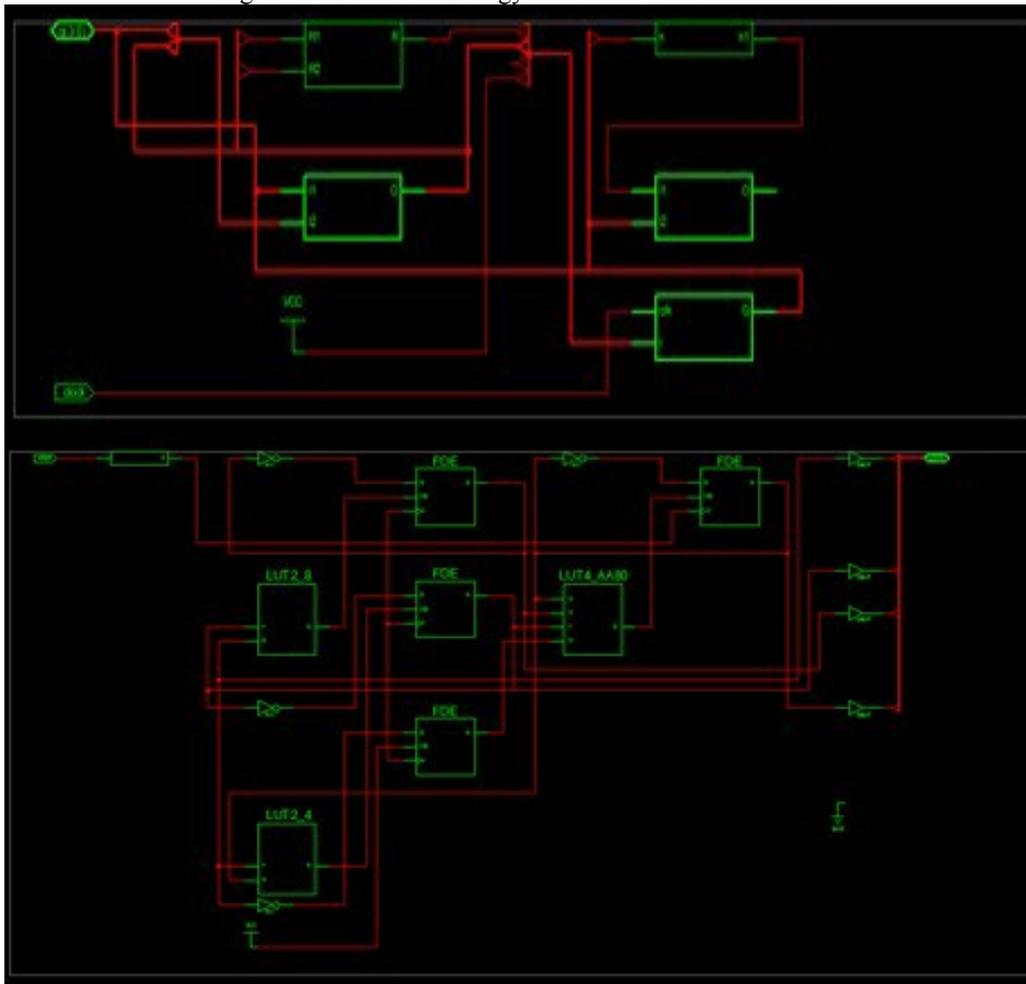
Fig. 2: RTL and Technology Schematics of a Counter.
