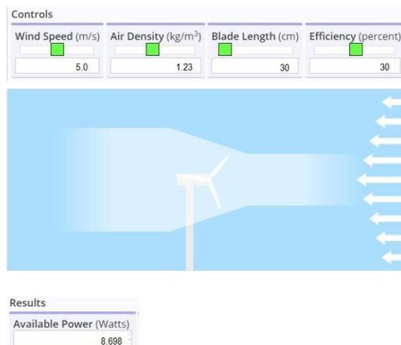
A simulation has been done for the estimated power calculation with the available wind velocity for the 5 bladed HAWT.
