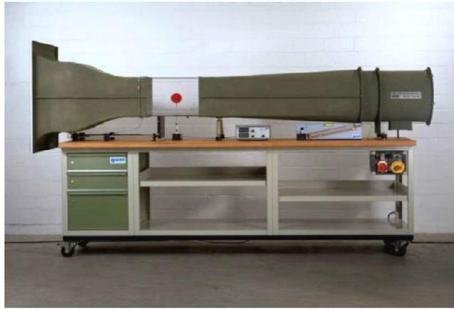
Fig. 2: Model of Wind Tunnel
