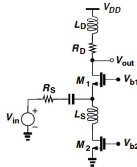
Fig. 2: Common-gate stage
