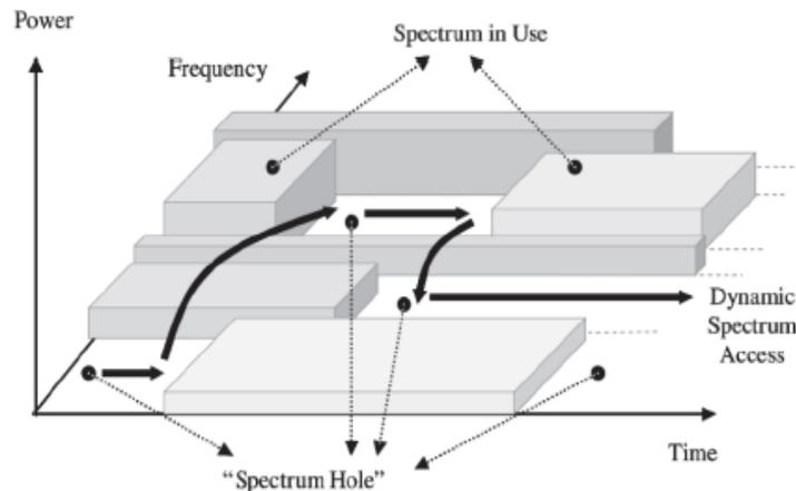
Fig. 1: Illustration of Cognitive Radio [2]
