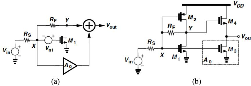
Fig. 5: (a) Noise-canceling LNA, (b) Implementation of (a)
