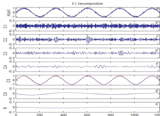
Fig. 3: Random White Gaussian Noise is added to input signal and EEMD is performed
