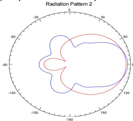
Fig. 5: Radiation pattern (Gain dB) of patch antenna with (Blue) and without (Red) metamaterial cover, showing improved directivity
