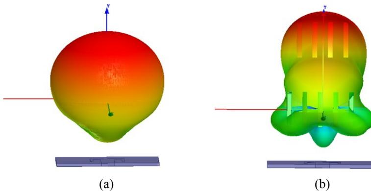
Fig. 6(a): 3D-polar plot showing directivity of a conventional patch without metamaterial cover, (b): with metamaterial cover.
