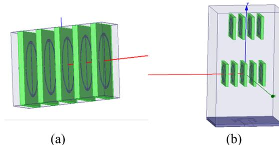
Fig. 3 (a) Array of metamaterial unit cells, (b) Array of metamaterial placed as a cover in front of patch
