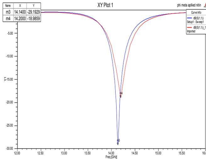
Fig. 4: S11 (dB) parameter of a patch antenna (Red), S11 (dB) parameter of patch antenna with metamaterial cover (Blue), showing resonance at ~14 GHz
