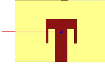
Fig. 2: A Microstrip Patch at 14 GHz.
