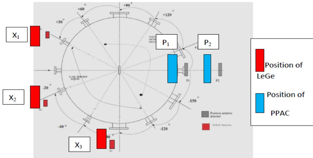
Fig. 13: Diagram shows the position of the detectors while performing the experiment.
