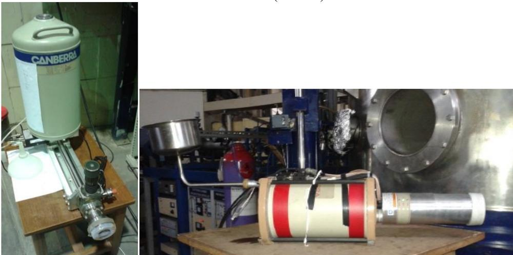
Fig. 11: Pictures of LeGe detectors, vertical on the left and horizontal on the right.
