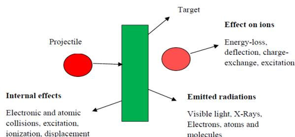
Fig. 1: Schematic representation of an ion-atom collision
