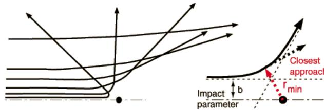
Fig. 3: Scattering of projectile by target at different scattering angles
