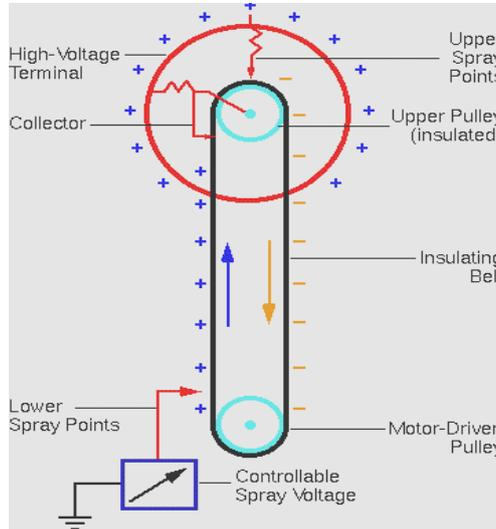
Fig. 7: Schematic diagram of the principle of a pelletron accelerator.
