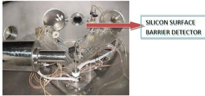
Fig. 14: Silicon surface barrier detectors are placed on the rotatable arms of the chamber to detect the scattered projectile.
