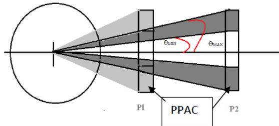
Fig.15: Change in measurable scattering angle with change in position of PPAC.
