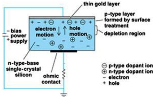
Fig. 12: Diagram showing principle of operation of a SSBD
