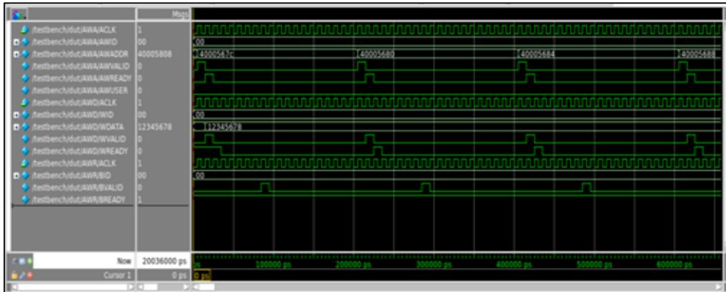
Fig. 5: AXI Write Channel signals
