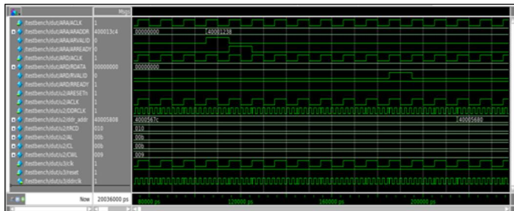
Fig. 6: AXI Read Channel Signals
