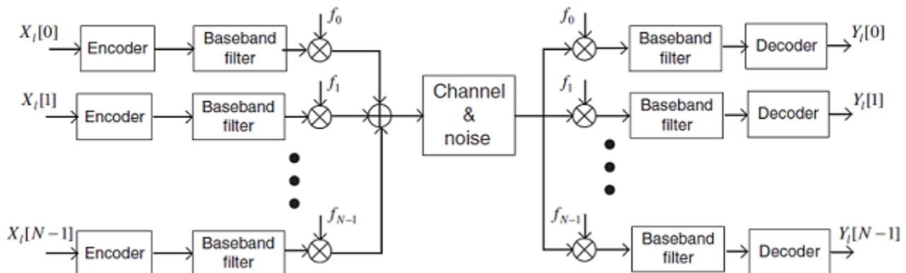
Fig. 1: Basic structure of multicarrier system
