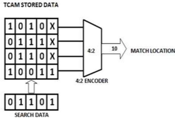
Fig. 5.2.1: Operation of 4 ×5-Tcam-Array
