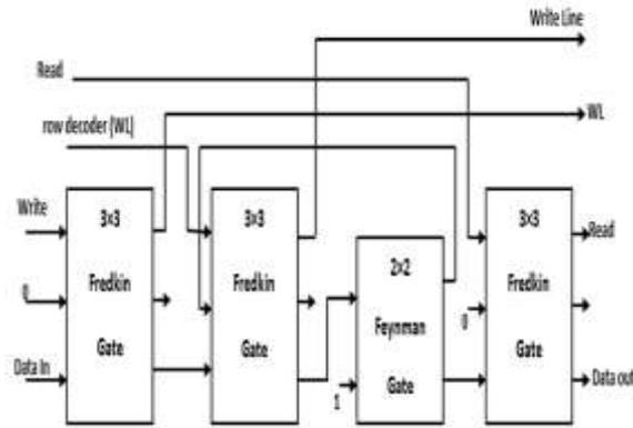
Fig. 3.2.2: Sram Cell Having Read/Write Signals
