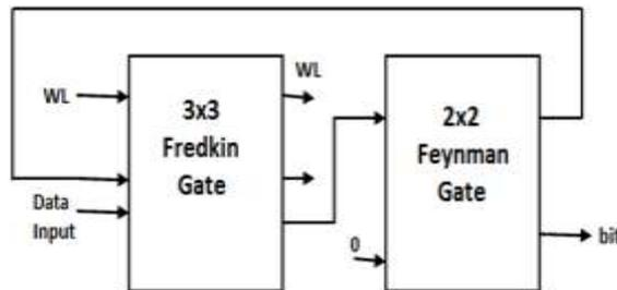
Fig. 3.2.1: Simple Sram Cell
