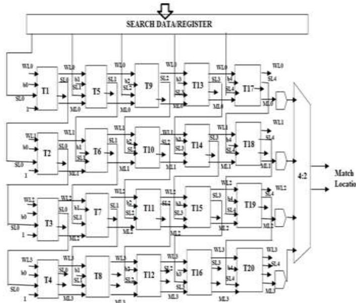
Fig. 5.1.1: Proposed 4x5-TCAM-ARRAY
