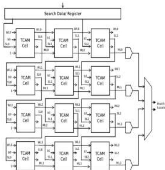
Fig. 4.2.1: Conventional 4 × 3-Tcam Array
